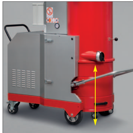
Progressive lowering of the collection bin
