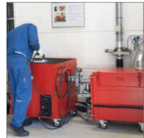
NA 250 Sheet steel without residual dust filter for use in plasma cutting
