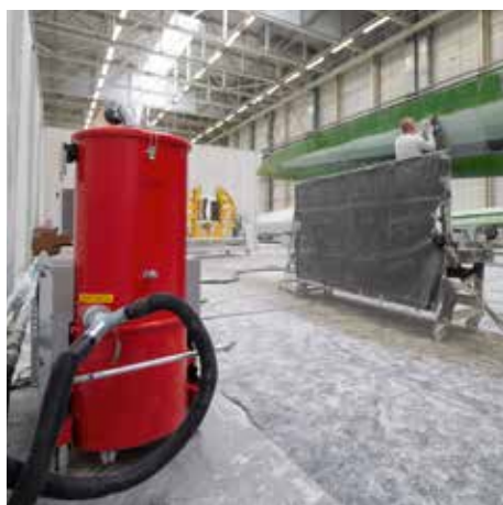
Tolmu imemine rootorilabade tootmisel GRP tolmust labade tootmine
