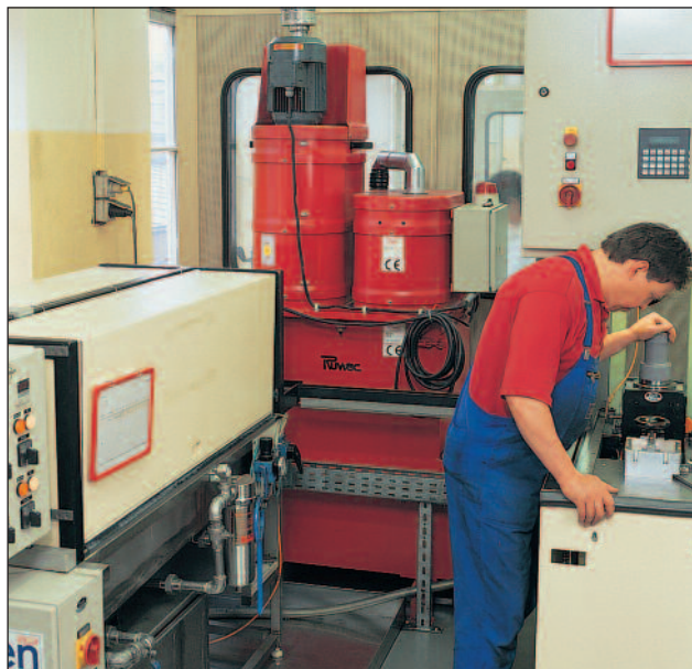
Standard vacuum cleaner with dome-type cyclone filter with additional oil mist cartridges.
